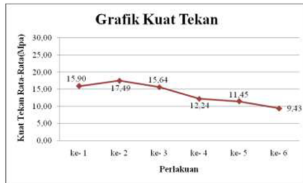
Figure 1. Paving Block Compressive Strength Chart (Source: Data Analysis, 2019)
